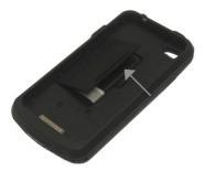
3. Lift the battery cover as shown in the figure above. Remove the existing battery. Reverse Steps 1-2 to install the new battery.
