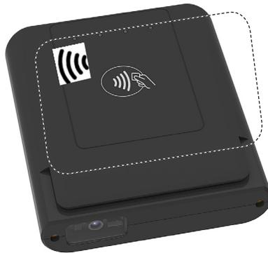
*Figure 10: Contactless Card Reader*
