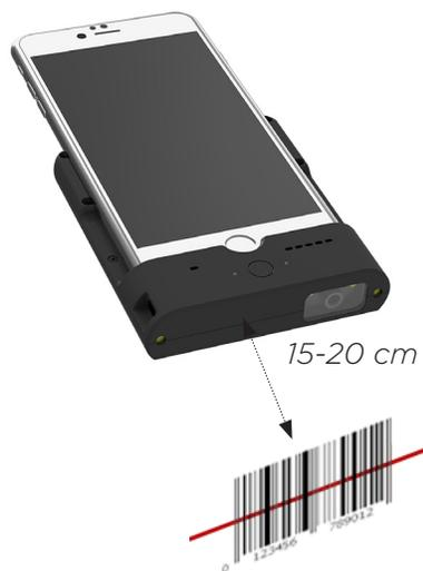
*Figure 7: 1D Barcode Scanning*
