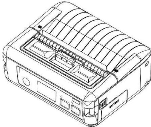
5. Slide locking lever to release battery as shown in the figure below
