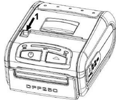
2. Lift the paper cover latch to open the paper cover as shown in the figure on the left.
