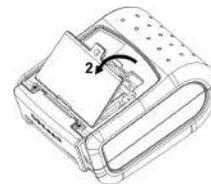
3. Lift the battery as shown in the figure on the right.
