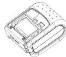
4. Detach the battery connector as shown in the figure on the right. Reverse Steps 1-4 to install the new battery pack.
